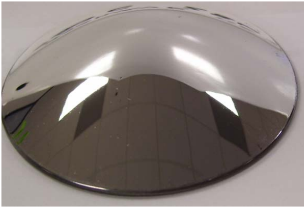
Figure 8. Secondary mirror coating #3 after 1000 hours at 250°C. No indications of failure.
