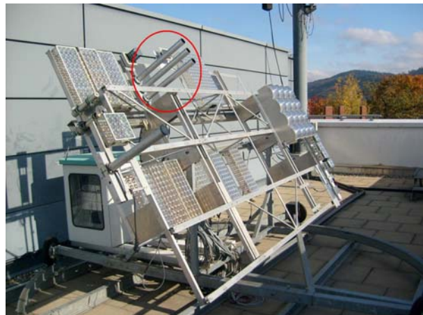
Fig. 1. Photograph of the CPV outdoor test set-up at the Fraunhofer ISE. The position of the three collimator pipes with underneath mounted isotype cells is marked with a circle.
